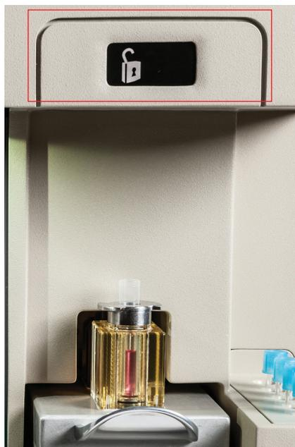
Fig. 7. Touch locking system screen.
