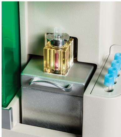
Fig. 5. Loading stage in the wash position.
