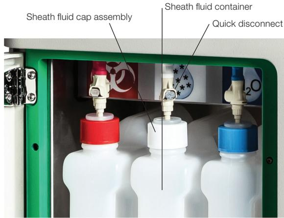
Fig. 29. Bulk fluidics with sheath fluid components noted.
