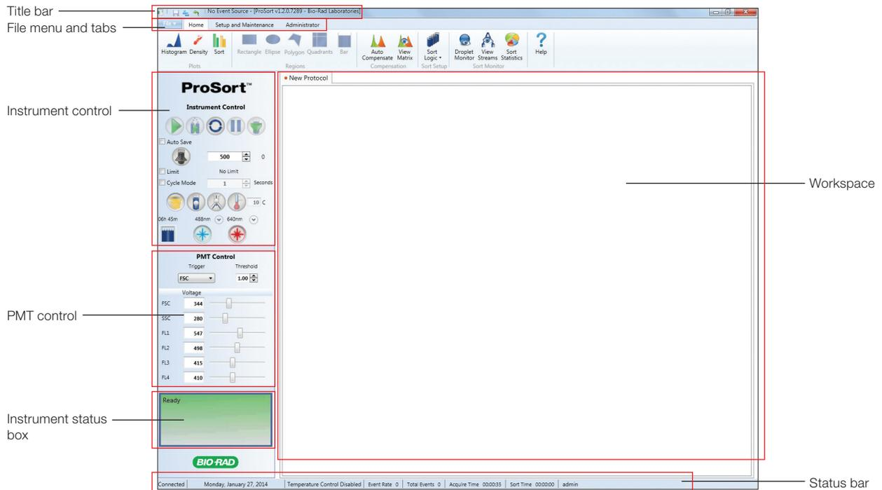
**Fig. 13. Main software window for user mode.**
