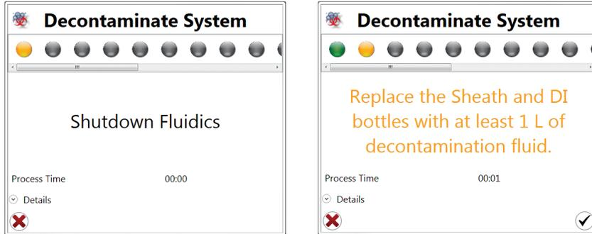
Fig. 130. Decontamination instructions to prepare the system.
