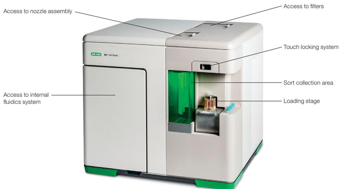
Fig. 1. Front view of the S3 system.
