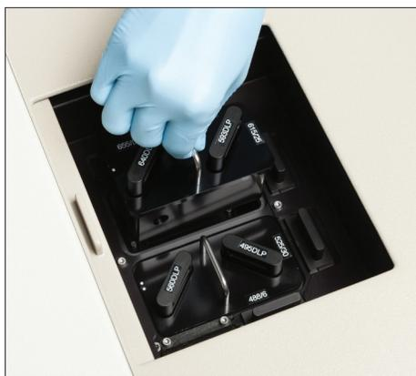
Fig. 69. Lifting an optical filter block.
