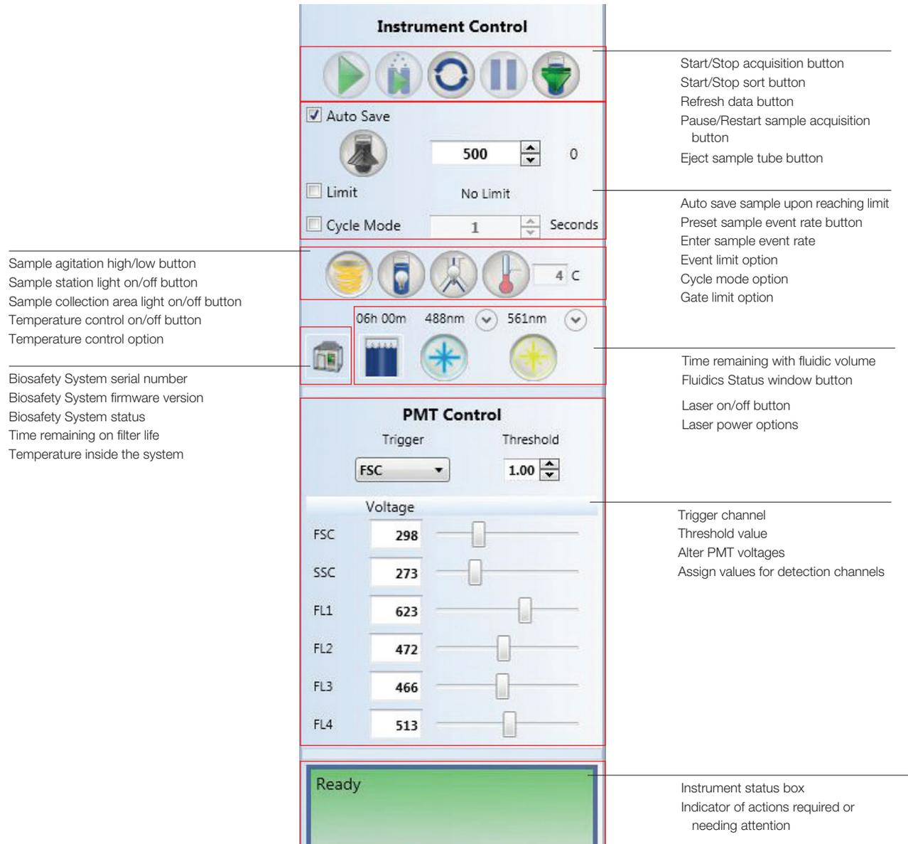
Fig. 16. Overview of instrument and PMT control panel.
