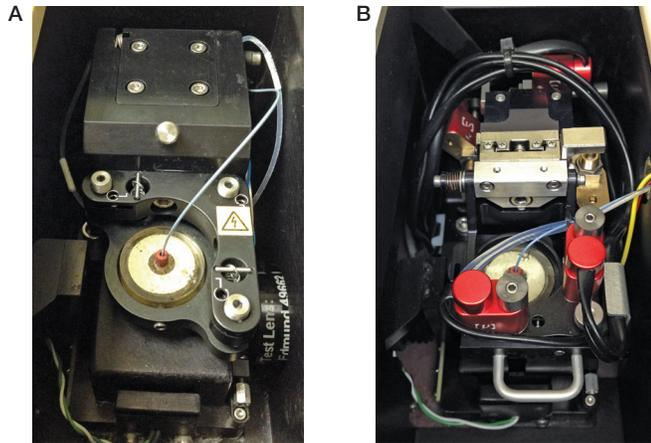
Fig. 8. Nozzle compartment containing the nozzle stage. A, Agilis System; B, AutoGimbal System.
