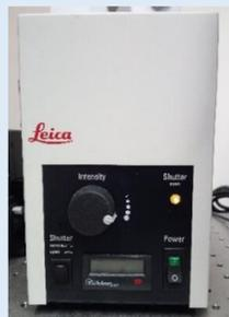
2 Microscope Power Supply CTR6000
