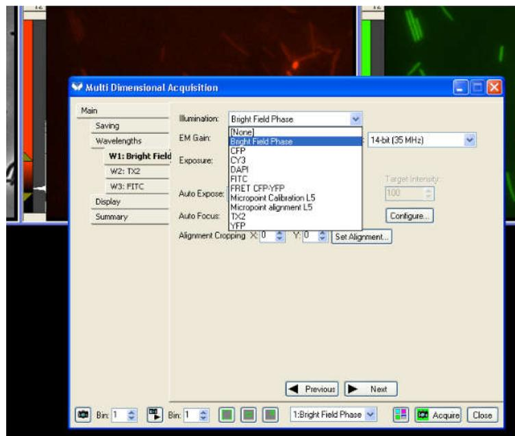
7. Select the adequate **Exposure Time**. Start small (200 ms) and increase if necessary to reduce bleaching (See Notes 3).
