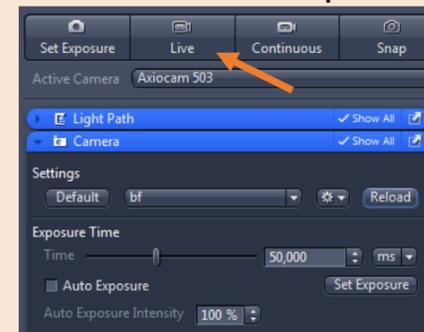
4 Focus the sample using SYCOP 3. Press Snap to acquire
