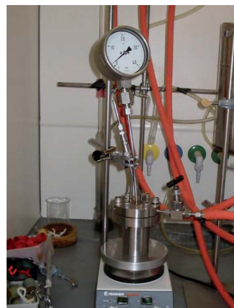
A stainless steel autoclave for hydrogenation reactions
