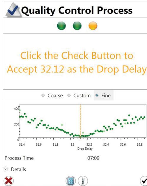
Fig. 6. Quality Control Process window showing calculated drop delay.
