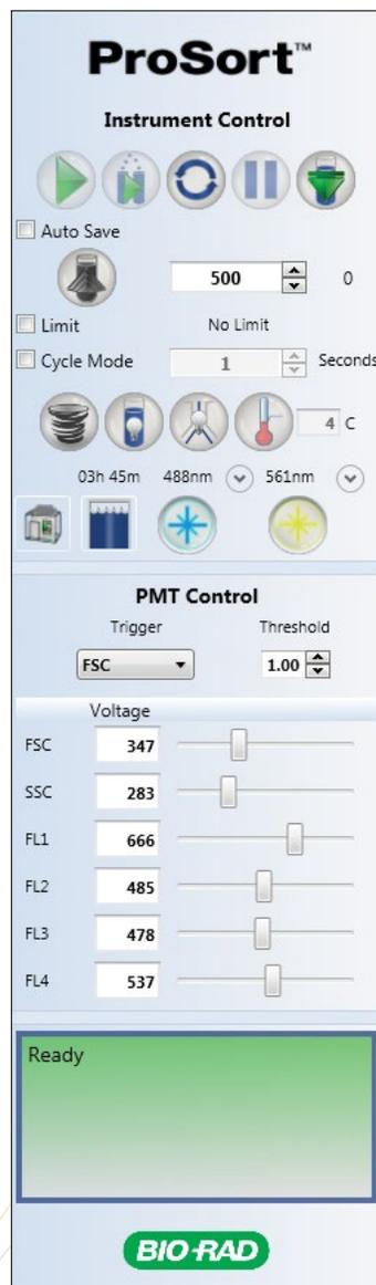
Fig. 8. Start and Stop buttons in the instrument control panel.
