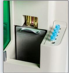
**8** When cleaning cycle is complete, move loading stage to Wash position
