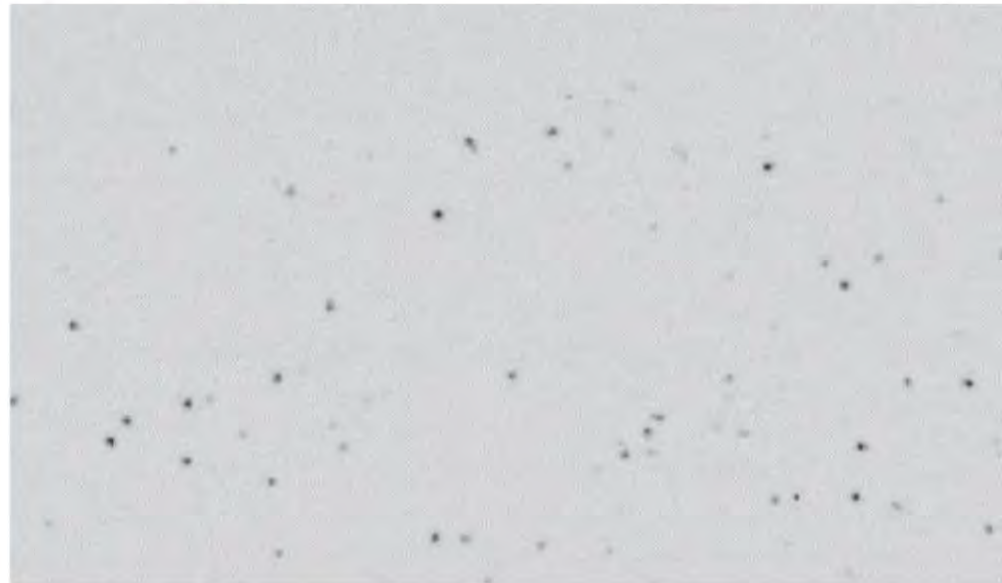
Single electron events in one frame from an active pixel sensor
