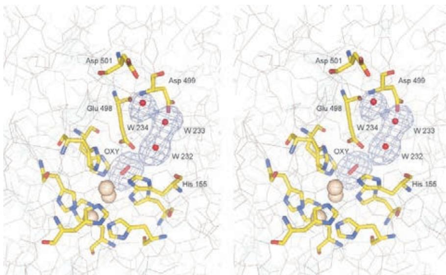
served in the fully oxidized structure of ascorbate oxidase (28), and the two T3 copper atoms are separated by 4.8 Å. This value is far closer to the value of 5.1 Å observed in the dithionite-reduced structure of ascorbate oxidase (29) than that of 3.7 Å in the corresponding oxidized structure.
