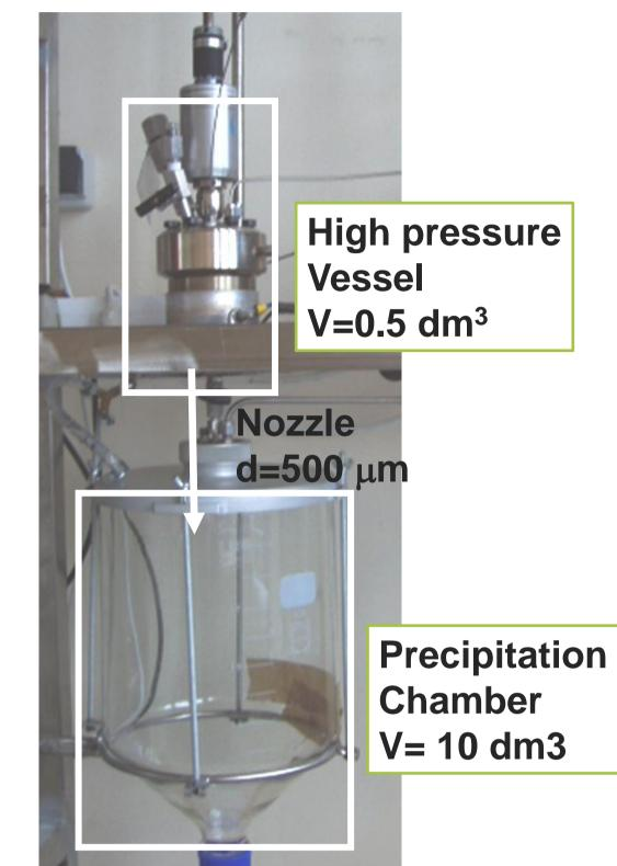
Supercritical fluids Technology Method: PGSS® Particles from Gas Saturated Solutions [1]
