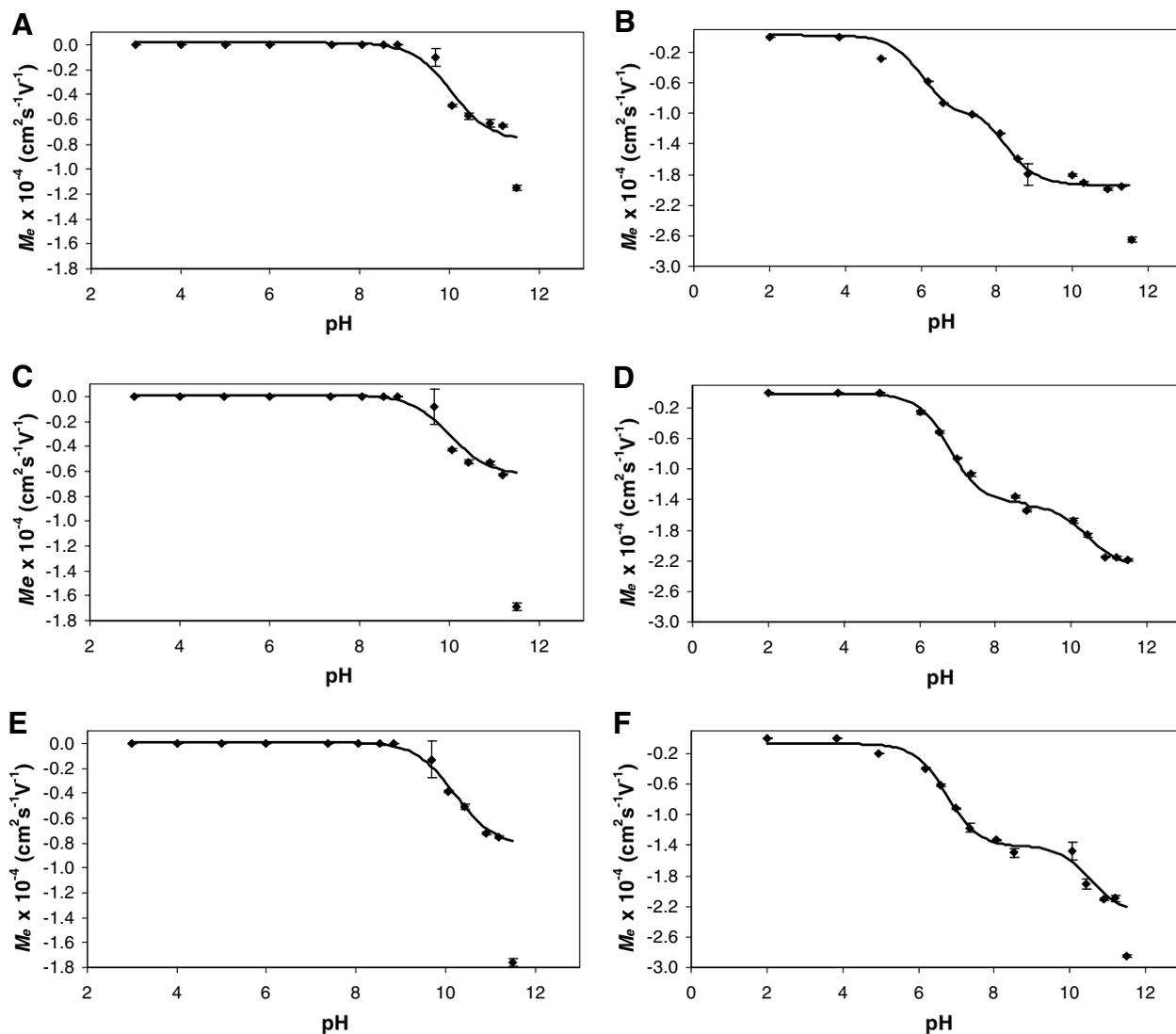
**Figure 2.** Ionisation curves ( $n = 3$ ) obtained for the test compounds by capillary electrophoresis (A, diosmin; B, diosmetin; C, hesperidin; D, hesperetin; E, naringin; F, naringenin).
