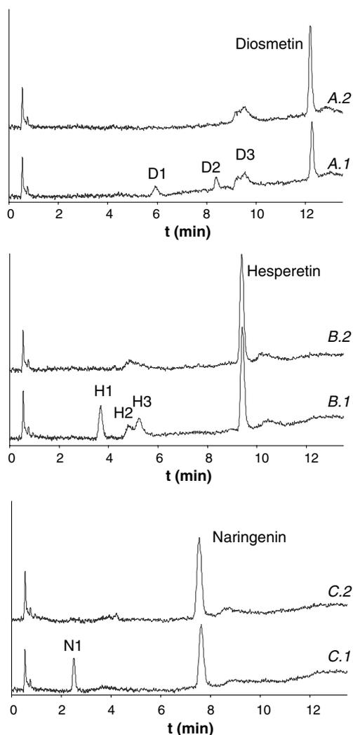
**Figure 4.** Metabolites of diosmetin, hesperetin and naringenin detected by HPLC in the apical solution after 120 min of apical loading (A.1, B.1, and C.1) and corresponding solutions after enzymatic hydrolysis (A.2, B.2, and C.2). Conditions as described in Experimental.
