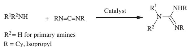
Figure 1. Catalytic addition of primary and secondary amines to carbodiimides.
